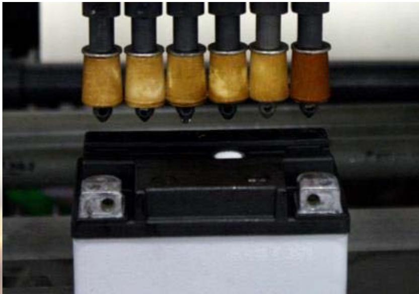
Precision filled to ensure saturation of entire glass mat area
