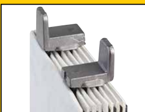
Electrolyte absorbed glass mats completely protect the plates for premier cycle service power and longer life.
